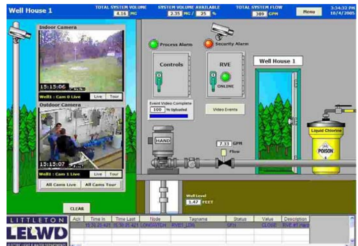
Figure 1: Video images on the HMI screen at the Littleton water department in Littleton, MA, allow operators to see what's happening in the well house and surrounding area.
