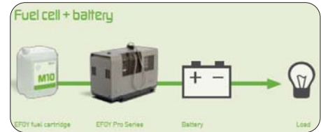
Figure 1: Operation of fuel cell and battery
